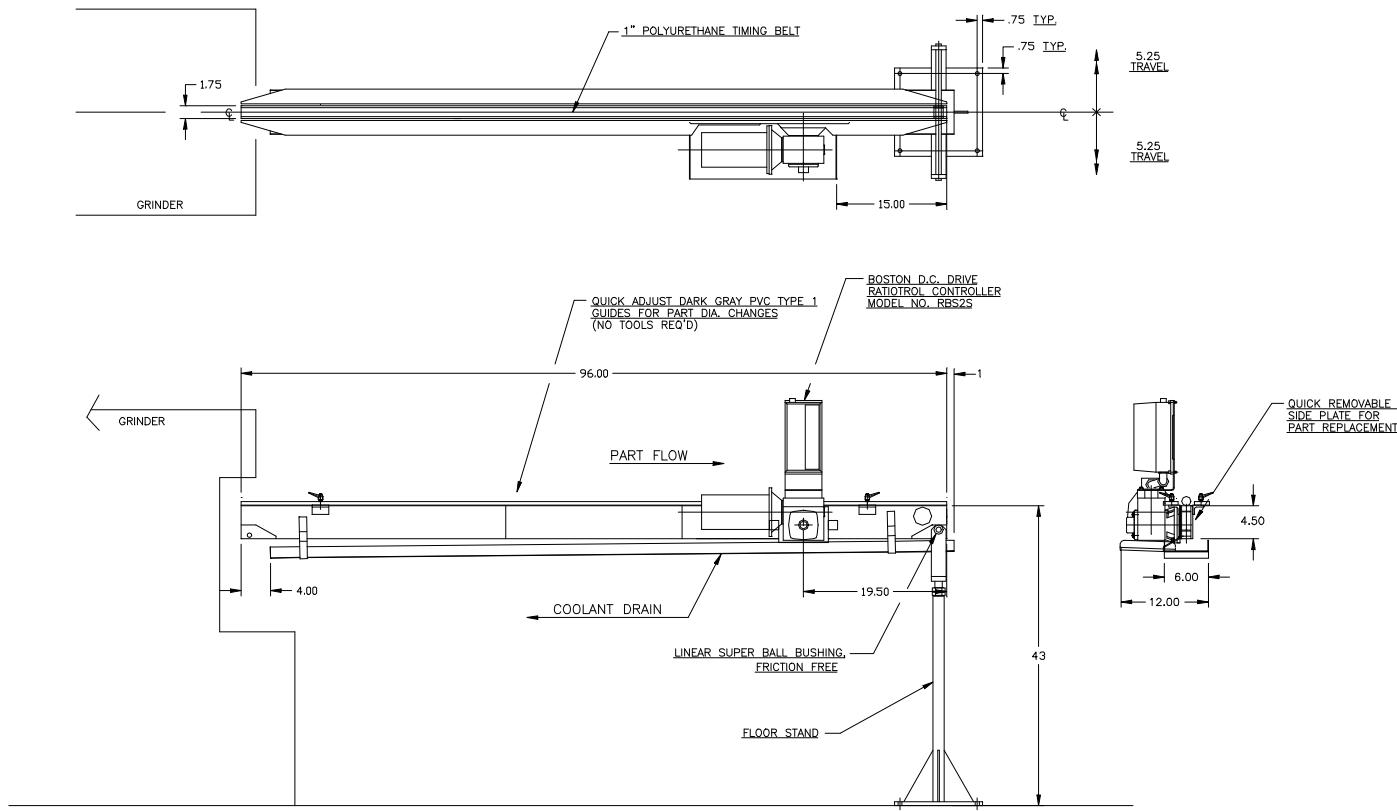
**APPLICATION:** Convey Steel Shafts from the workrest of a Centerless Grinder.
