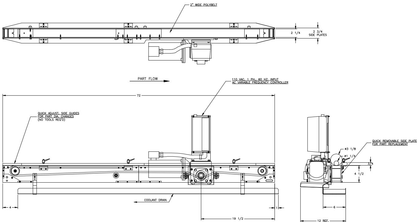
**APPLICATION:** Convey Pinion Shafts to the workrest of a CINCINNATI Model 325 Centerless Grinder.
