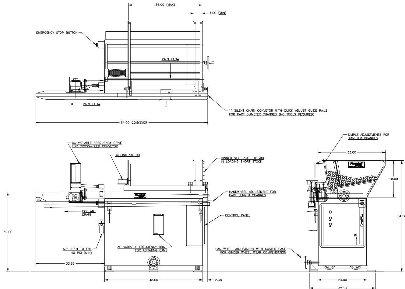
**APPLICATION:** Feed from a manually loaded, floor mounted magazine. Shafts will be fed in a continuous stream and escaped one at a time onto a front mounted cross-feed conveyor. The conveyor will translate parts in a continuous stream to the workrest of a CINCINNATI centerless grinder.
