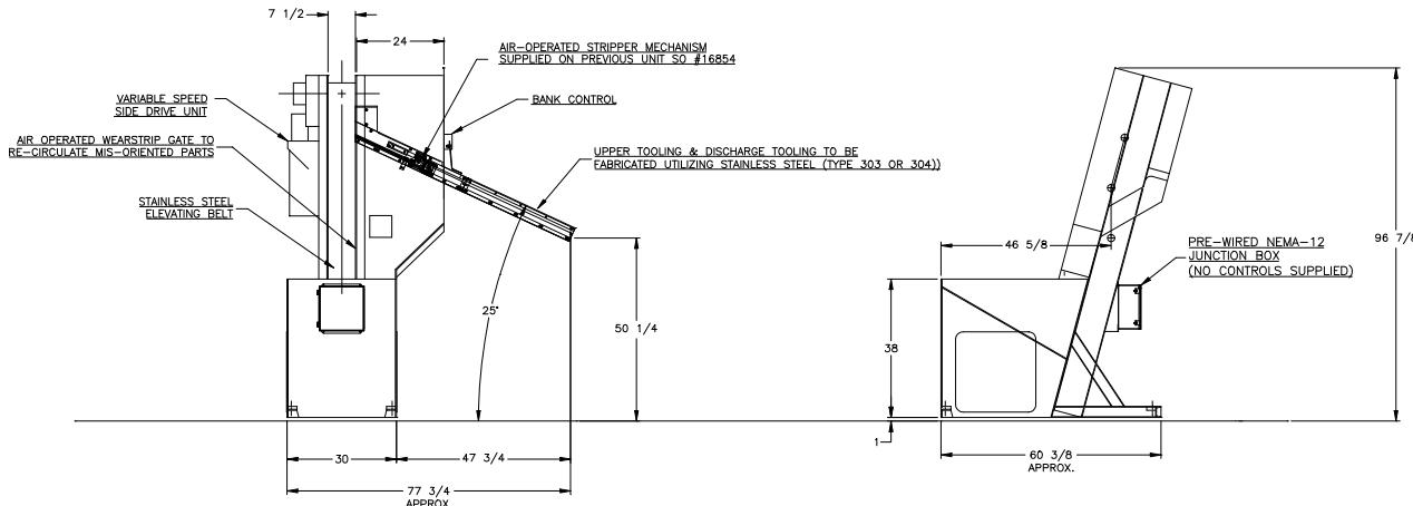
**APPLICATION:** Feed from a random loaded, floor mounted hopper. The parts will be elevated from the hopper via a cleated belt and discharged in a continuous stream at 25°.
